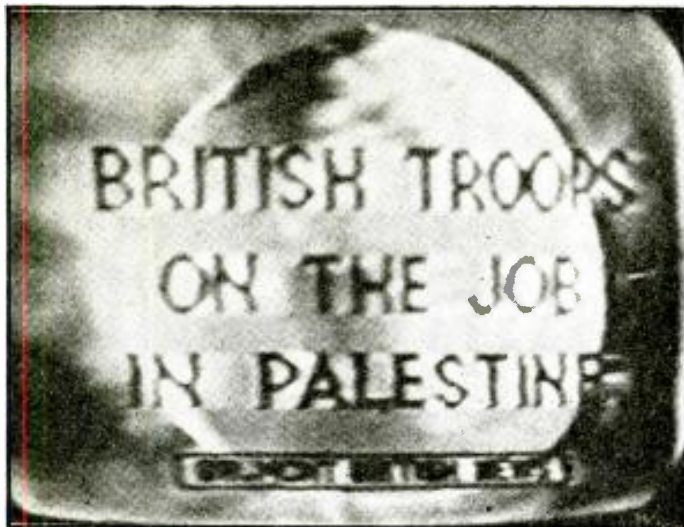
Fig. 4. Still another photograph showing the effects of oscillator detuning, and inadequate frequency response in the I.F. circuits.
