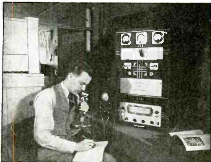
Great Smoky Mountains National Park Headquarters radio station at Gatlinburg, Tenn., may soon have the above-type 50-W. Fire Dispatcher's radiophone.
