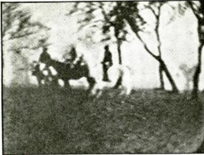
Fig. 2. This curious effect results from the combination of incorrectly-tuned oscillator, and inadequate frequency response in the I.F. circuits.
