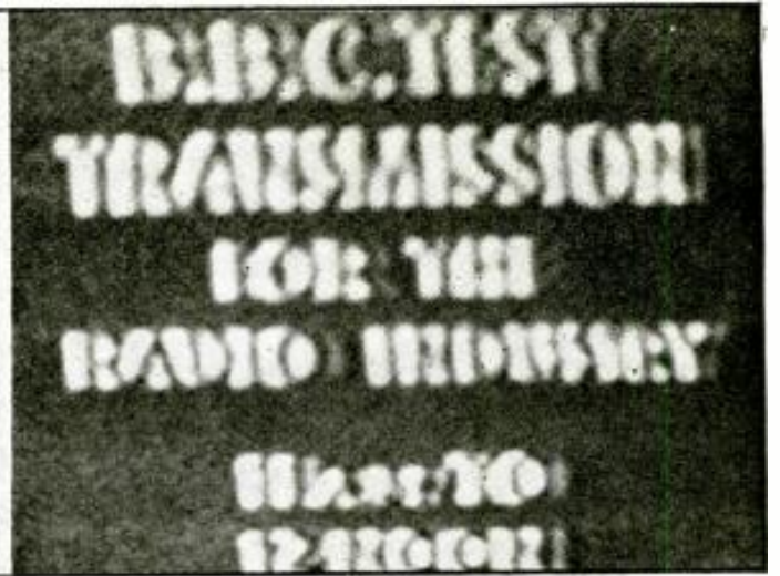
Fig. 3. This photograph depicts effects similar to those shown in Fig. 2, these are, incorrect tuning of the oscillator, and low I.F.-circuit frequency response.
